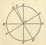
the latitude of the place becomes known. Thus in the figure let the circle be a meridian section of the celestial sphere, P the pole, Z the H zenith, Q the equator, S the sun, and HH the horizon. The arc SH' is the altitude of the sun, SQ is its declination, and ZQ is the latitude of the place of observation A. Let h be
